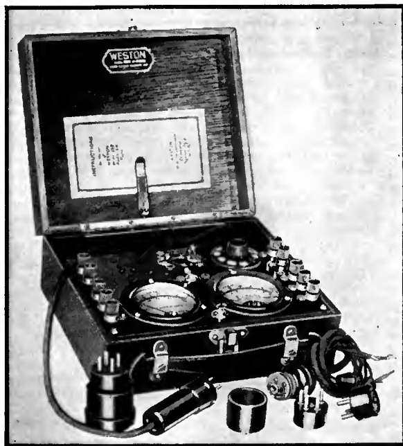
The Weston tube-checker is an excellent piece of shop equipment for the dealer-serviceman. Any 4 or 5 prong tube may be tested with this set
